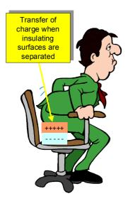
Figure 1 The ESD charging process
